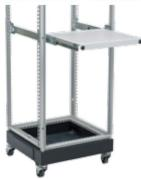
Frame Pull-Out Shelf allows easy access to shelf-mounted devices. The shelf is 16 gauge steel with 12 gauge steel supports. The entire assembly is finished with RAL 7035 textured gray polyester powder paint. The shelf mounts to the front and rear frame uprights. Load rating is 110 lb. (50 kg).
